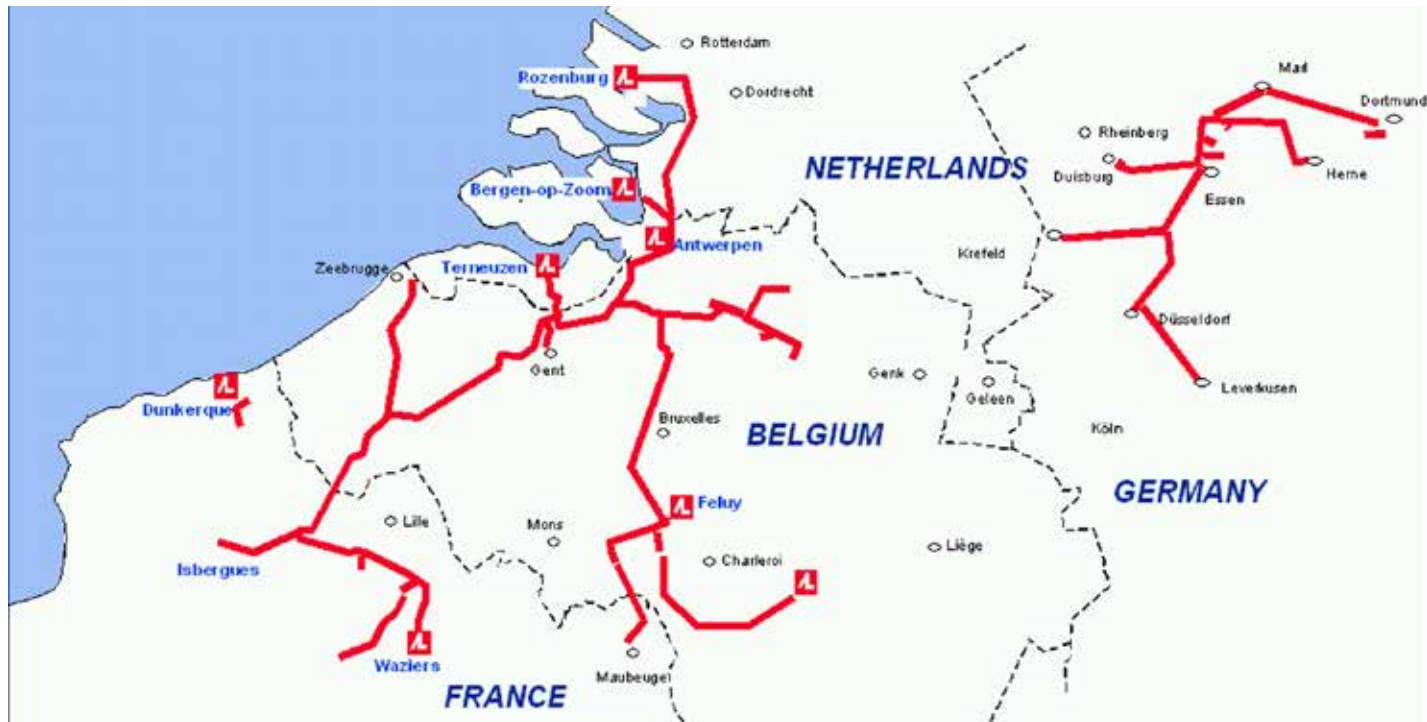
The hydrogen piping network in Belgium and its neighbouring countries - Photo courtesy of Air Liquide
