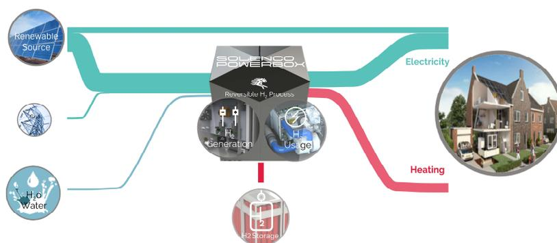
At night or when there is a lack of electricity, the stored hydrogen can be transformed by the reversible PEM fuel cell side into electricity and heat. The electricity goes to appliances and the heat is used for low temperature heating systems as well as sanitary water heating.
